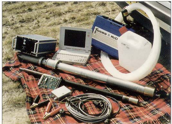
Fig. 4. Cone Pressuremeter equipment spread
