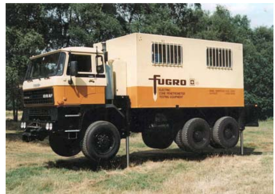
CPT rig used to push in “Vibro-Cone”
