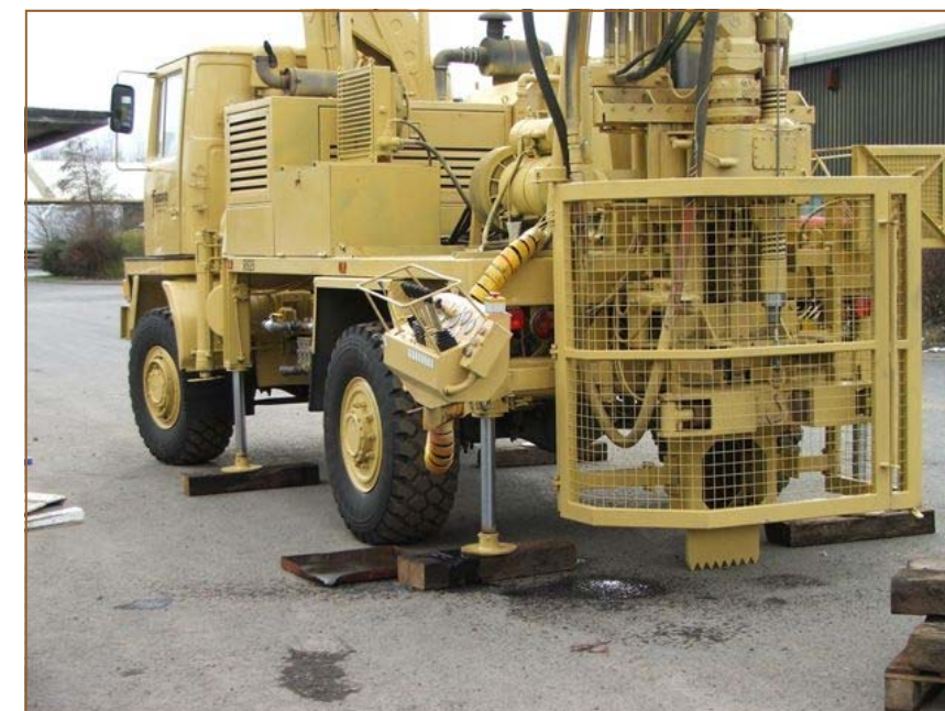
“Drilling rigs are required by HSE to have adequate guarding. Under new CDM regulations it becomes the clients' responsibility to ensure their drilling sub-contractors comply”
